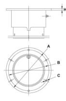
H = 7mmA = Ø183mm B = Ø165mm C = 4 holes Ø7mm
